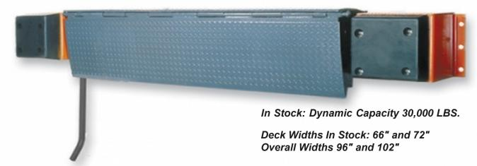
Perma Tech Mechanical Edge of Dock BLE Series provides an operating range of 5" above and 5" below dock, with a minimum lip projection of 12 3/4" and an overall span of 27 3/4". Broad center-plate and lip are constructed of 55,000 lb. minimum yield steel tread plate. The Perma BLE Series Levelers are exclusively equipped with 3 formed steel gussets, providing 30,000 lbs. of structural support in the stored position.
